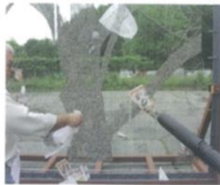
Photo 4: Debris being introduced to the tapestry.
